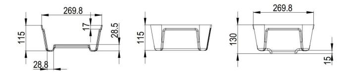
Our hydroponic gutter are composed of Head + Mid + End, which designed to easily connect multiple gutter part together, end-to-end. There are male and female end designs, the female end underlap nests under the male overlap for a snug fit when connecting trays. Use suitable ABS adhesive to attach the male end overlap firmly on top of the female end. This allows for a unlimited length level growing surface across multiple tray pieces.
