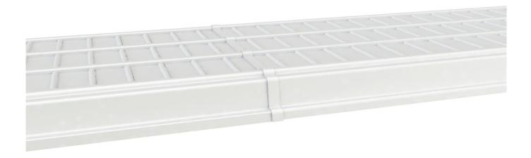
Infinity Trays are composed of Head tray + Mid tray + End tray, which designed to easily connect multiple trays together, end-to-end. There are male and femal end designs, the female end underlap nests under the male overlap for a snug fit when connecting trays. Use suitable ABS adhesive to attach the male end overlap firmly on top of the female end. This allows for a unlimited length level growing surface across multiple tray pieces.
