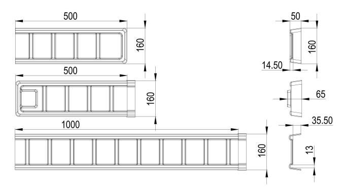
Our hydroponic gutter are composed of Head + Mid + End, which designed to easily connect multiple gutter part together, end-to-end. There are male and female end designs, the female end underlap nests under the male overlap for a snug fit when connecting trays. Use suitable ABS adhesive to attach the male end overlap firmly on top of the female end. This allows for a unlimited length level growing surface across multiple tray pieces.
