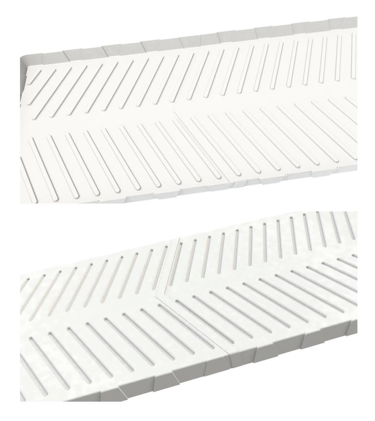
Infinity Trays are composed of Head tray + Mid tray + End tray, which designed to easily connect multiple trays together, end-to-end. There are male and femal end designs, the female end underlap nests under the male overlap for a snug fit when connecting trays. Use suitable ABS adhesive to attach the male end overlap firmly on top of the female end. This allows for a unlimited length level growing surface across multiple tray pieces.
