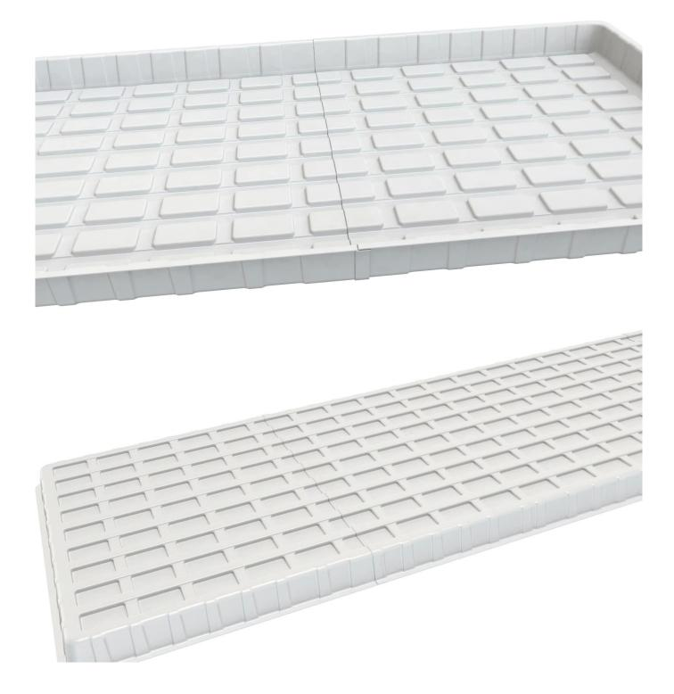
Infinity Trays are composed of Head tray + Mid tray + End tray, which designed to easily connect multiple trays together, end-to-end. There are male and femal end designs, the female end underlap nests under the male overlap for a snug fit when connecting trays. Use suitable ABS adhesive to attach the male end overlap firmly on top of the female end. This allows for a unlimited length level growing surface across multiple tray pieces.
