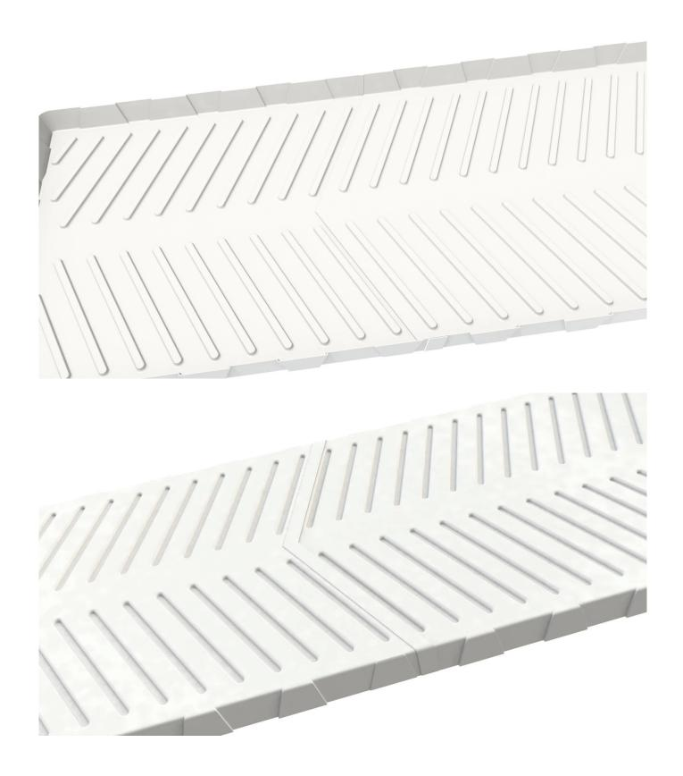
Infinity Trays are composed of Head tray + Mid tray + End tray, which designed to easily connect multiple trays together, end-to-end. There are male and femal end designs, the female end underlap nests under the male overlap for a snug fit when connecting trays. Use suitable ABS adhesive to attach the male end overlap firmly on top of the female end. This allows for a unlimited length level growing surface across multiple tray pieces.
